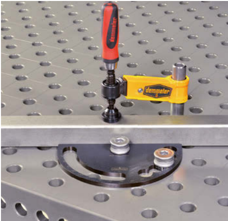
Fixed setting out in 15° increments (0° - 60°) and continuous 0° - 90°
