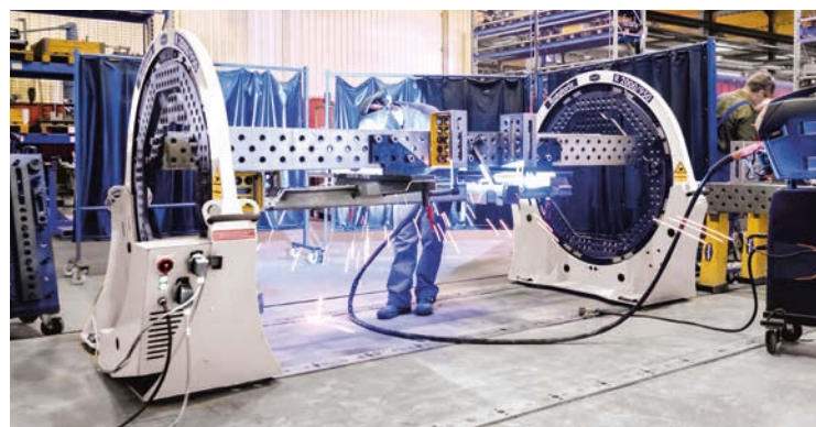
Rotatorix® with frequency-controlled drive on a DEMMELER foundation track system for work pieces of varying lengths
